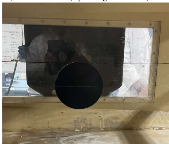
Fig 11. Side view of cylinder placed in testing section of low-speed wind tunnel in UCD Mechanical Engineering Lab.
