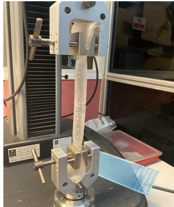
Figure 29: Prototype 2: Pull-to-failure set up for nonstandard investigatory tests of defective prototypes.
