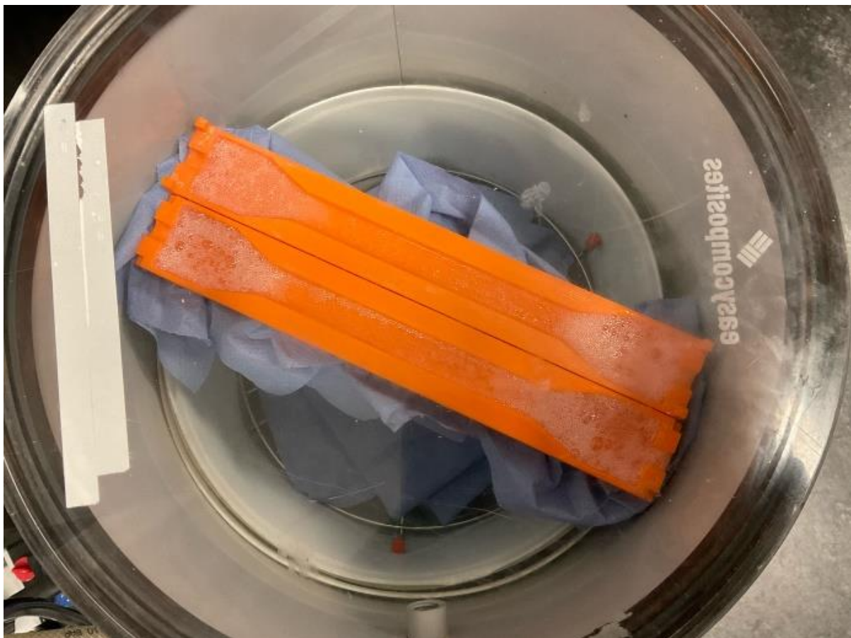
Figure 22: PLA moulds filled with Sylgard-184 in vacuum chamber for second round of degassing stage.
