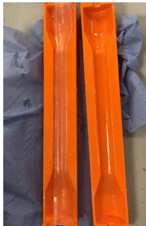
Figure 32: Prototype 1 full model - half model due to leaking between two moulds interface.
