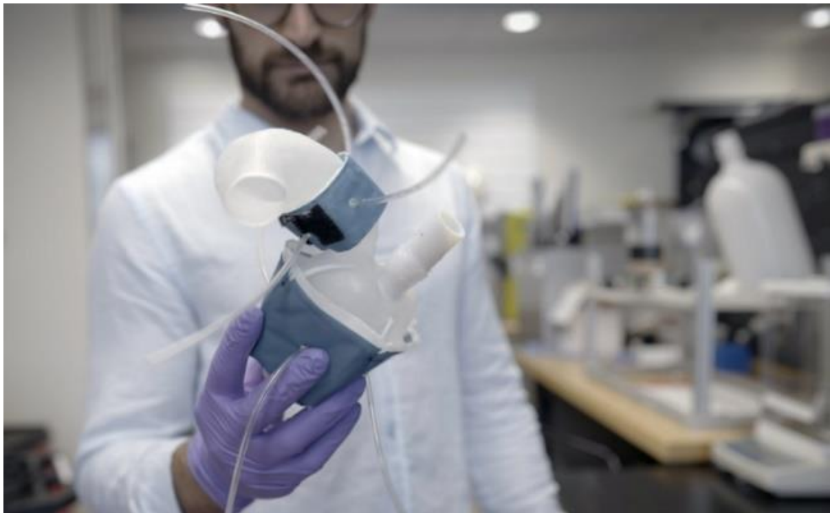
Figure 58: 3D Printed bionic custom heart made in MIT Laboratory for heart valve testing [2].
