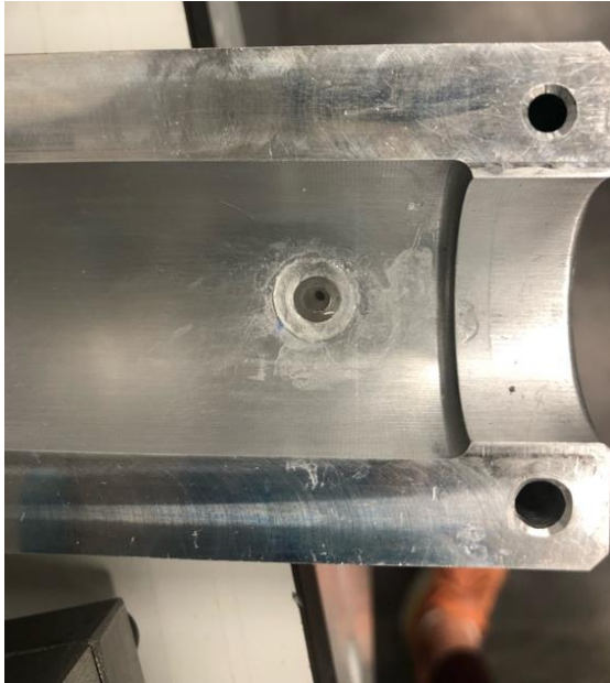
Figure 53: Plug glued to aluminium mould that allows for insertion of syringe with luer-locking adaptor. Inlet site for Sylgard-184 introduction.
