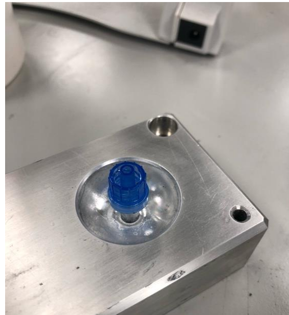
Figure 52: One way valve attached to injection site to prevent leakage of material when syringe removed.
