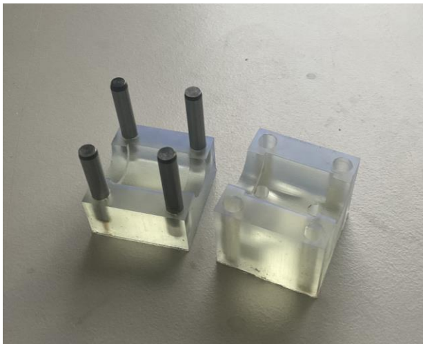
Figure 19: Iteration 3, utilizing dowl pins to align the moulds.
