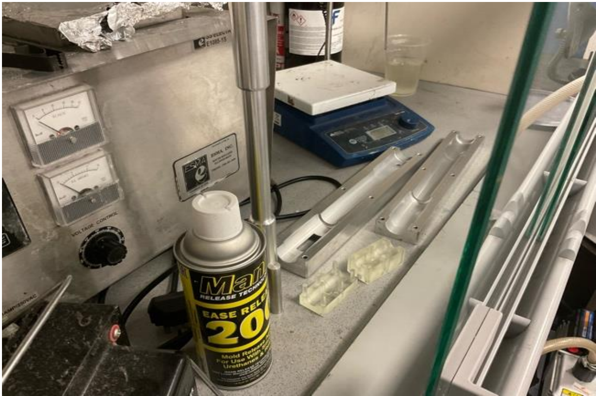
Figure 25: Ring and model moulds/mandrels left to dry in fume cupboard after applying Inhibition Agent (Resin prints) and Mould Release.
