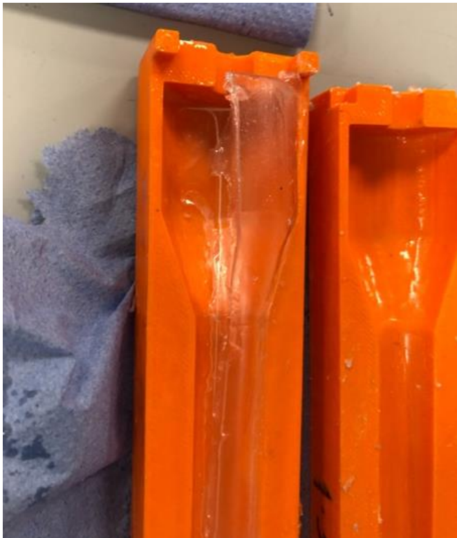
Figure 31: Prototype 1, failed due to leakage and insufficient sealing of mould interfaces.
