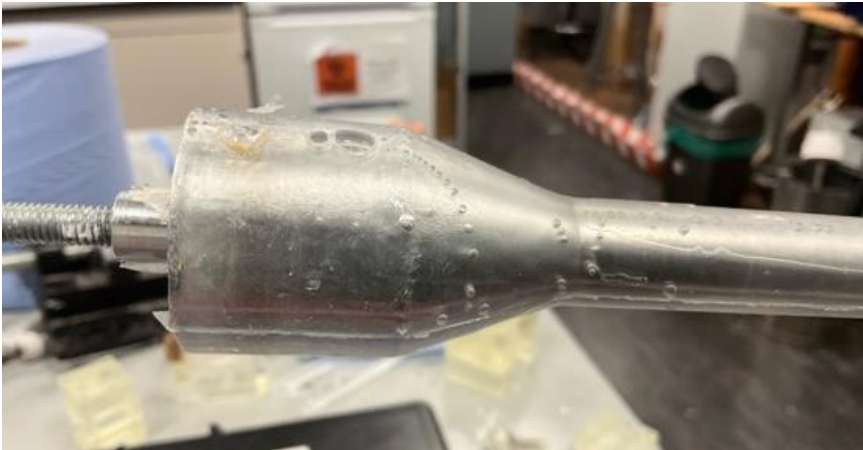
Figure 35: Defects of Prototype 2 shown: bubbles from poor Sylgard-184 degassing and introduction into mould. Trapped air bubbles, seamline, and markings from surface of PLA mould.
