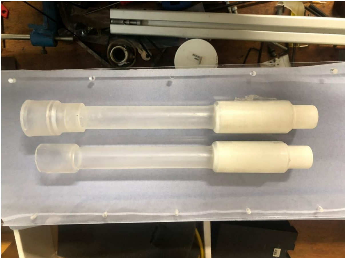
Figure 36: Two final models to be placed in right heart simulator with adjusted end attachments due to fragility of Sylgard-184. Bottom was cured at 100 °C and top at 21 °C.
