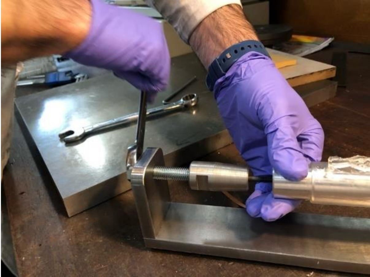
Figure 26: Splitting of mandrel to release model.
