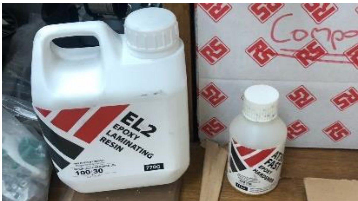
Figure 20: RS EL2 Laminating Epoxy Resin used for improving surface finish of mould surface.
