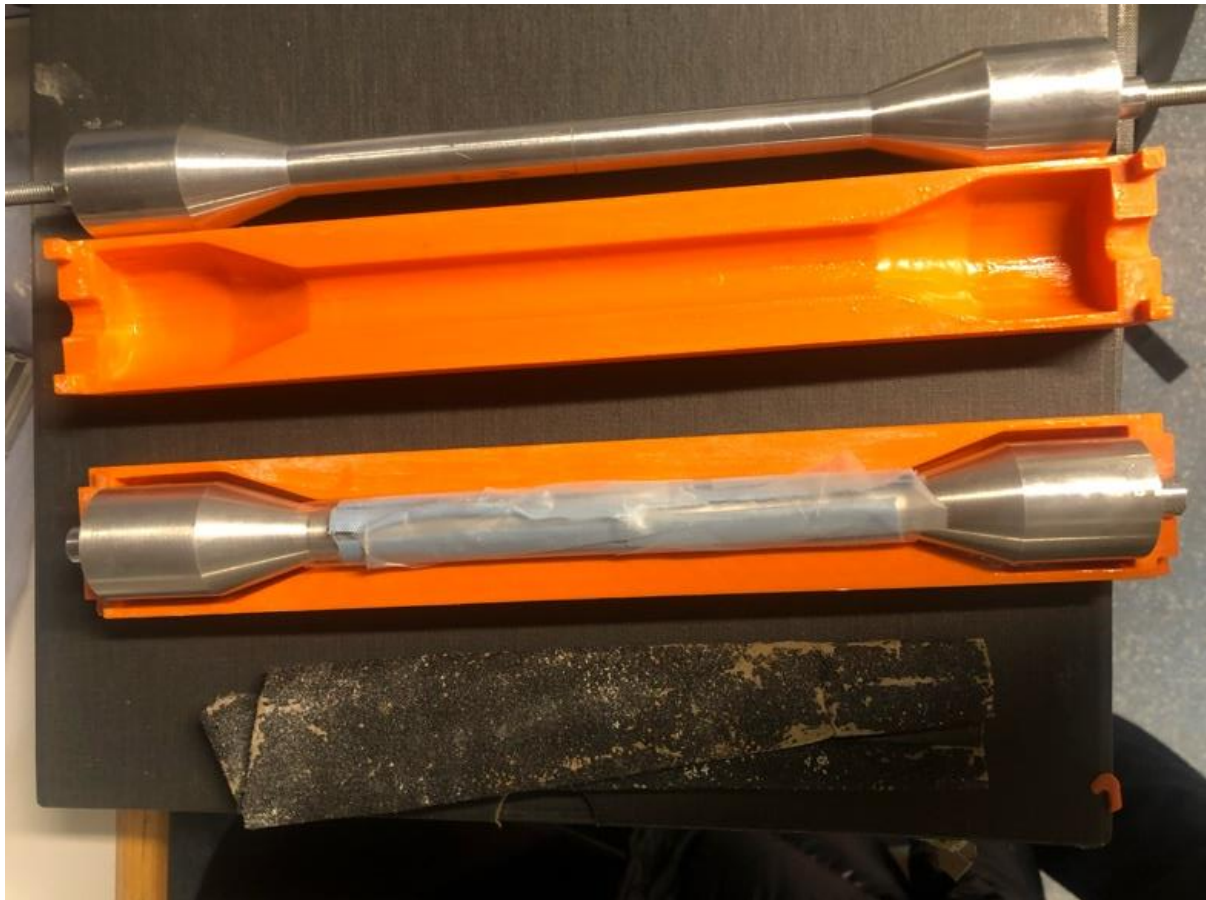
Figure 21: Plastic sheet around mandrel used to press epoxy-filler onto surface for smoother finish.
