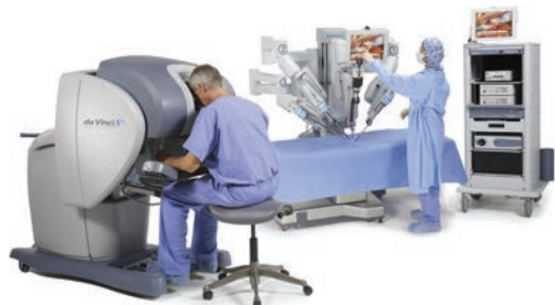
In performing robotic surgery, the physician uses controls at a console to maneuver the robotic instruments, while viewing high-definition, 3D images of the surgical site.
