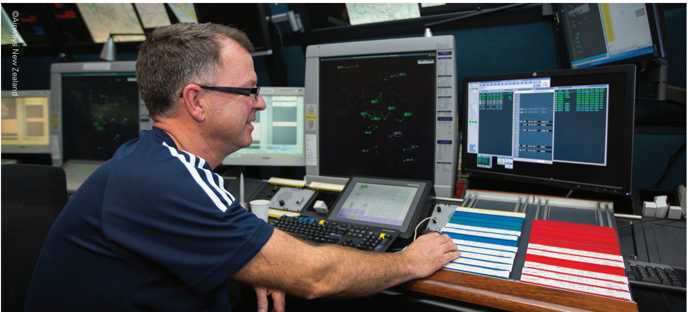
An Airways radar controller uses the CFM/AMAN solution, now in operation for flights into Auckland, to manage traffic bottlenecks and reduce airborne holding. Photo credit: Airways New Zealand
