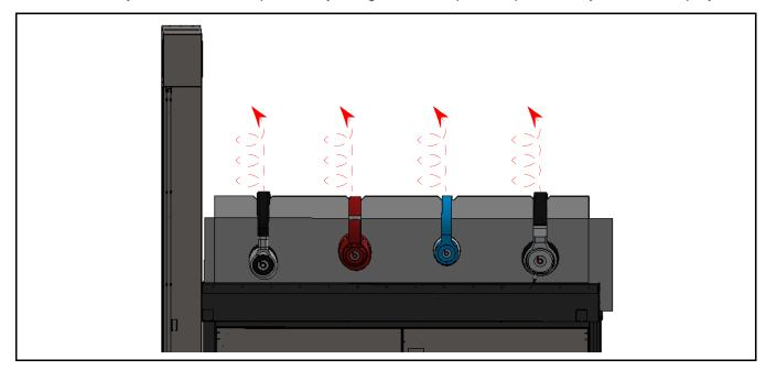
4. Make sure all of the LEDs on the main base unit and the lightbox are illuminated.
