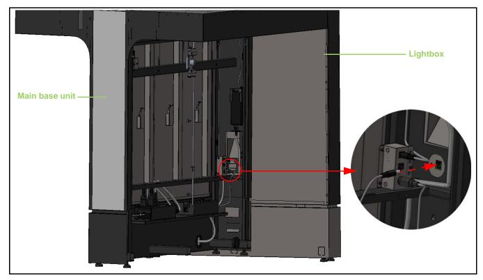
4. Insert the security screw through the main base unit and into the lightbox.
