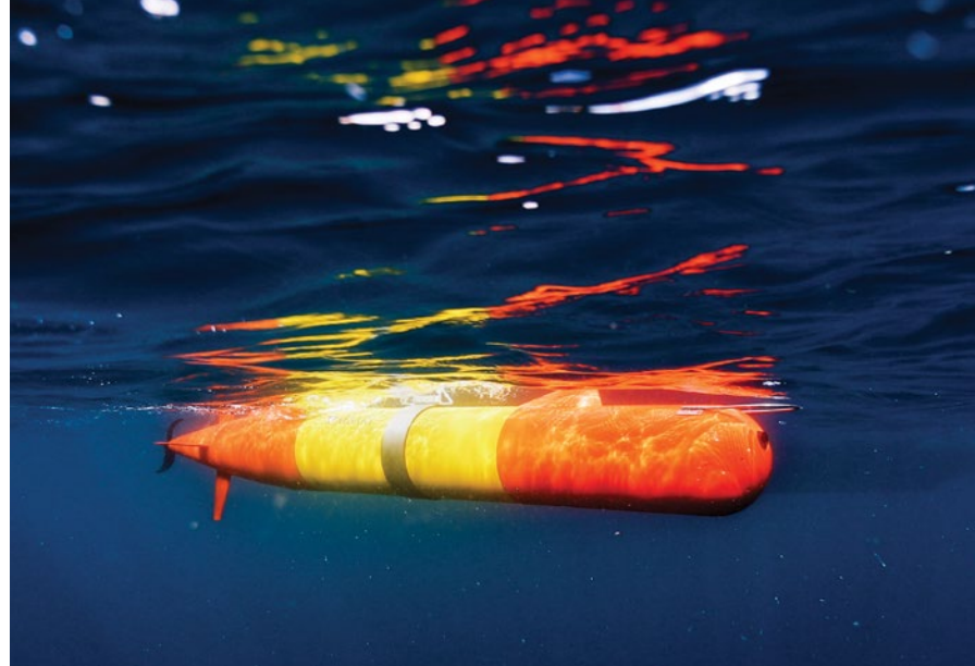
The Monterey Bay Aquarium Research Institute’s autonomous underwater vehicles can prowel water bodies for signs of harmful algal blooms. They take water samples and even do onboard chemical analysis.
