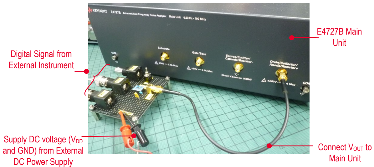
Figure 3. Photo of connection between evaluation PCB and E4727B Main Unit
