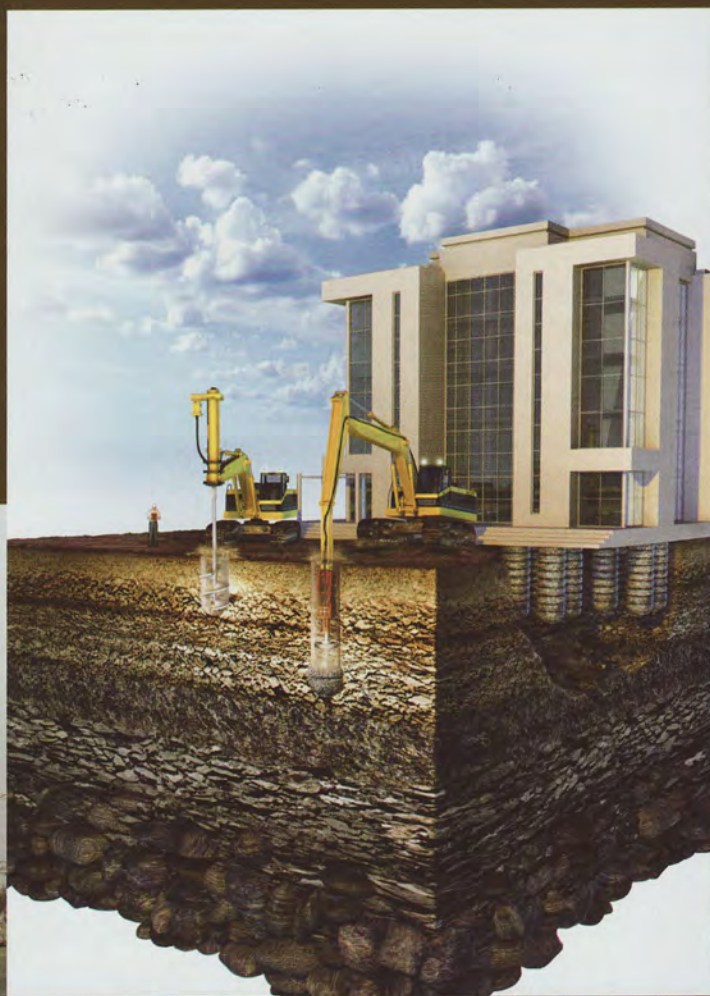
The rig on the right is demonstrating the Impact System as the aggregate poured into the cavity is compacted and forced downward and outward to create lateral pressure on the surrounding soil, doubling its bearing capacity.
