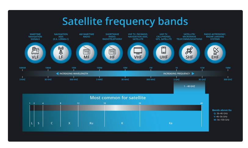
Today's satellites mostly operate in radio bands between 30 MHz and 40 GHz, and different sections of that "bandwidth" have been grouped like this:
