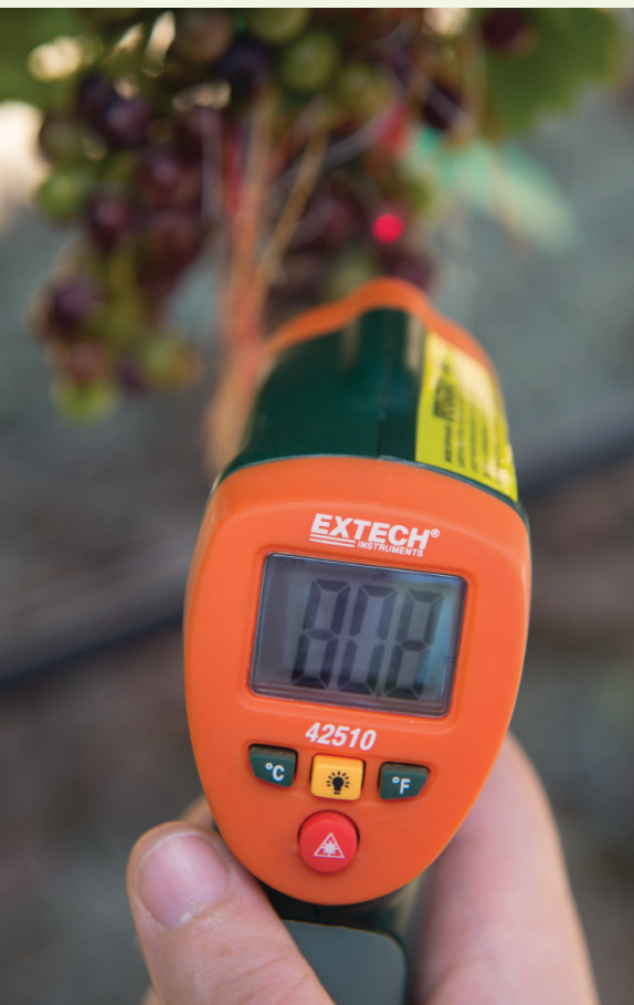
Above: Laurent Deluc uses fine color-coded threads to tag tiny grape berries. Below: An infrared thermometer takes the temperature of ripening grapes.
