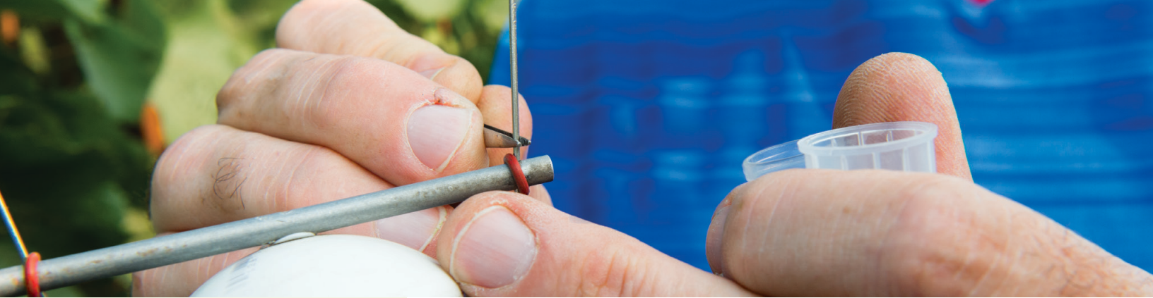
Above: Using tweezers, Walt Mahaffee removes stainless steel pins from a spore trap. He'll analyze them back at the lab to see if powdery mildew adhered to them. Left: Mahaffee checks the solar power connection to a spore trap.
