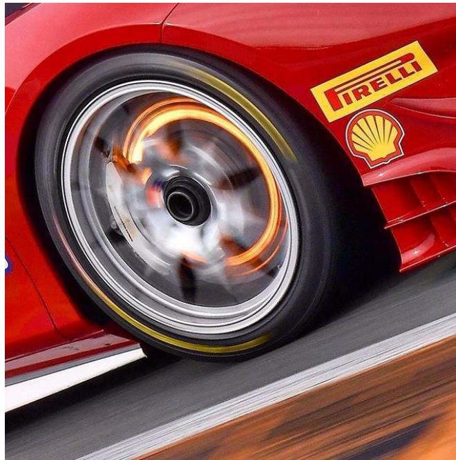
Figure 6: Carbon Ceramic Brakes glowing during heavy braking [10]
