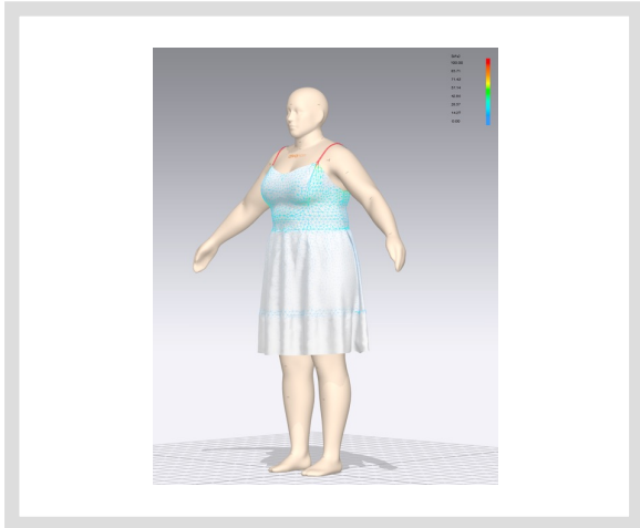
*Stress map displays the pressure of the fabric per section resulting from a tight-fitting garment
