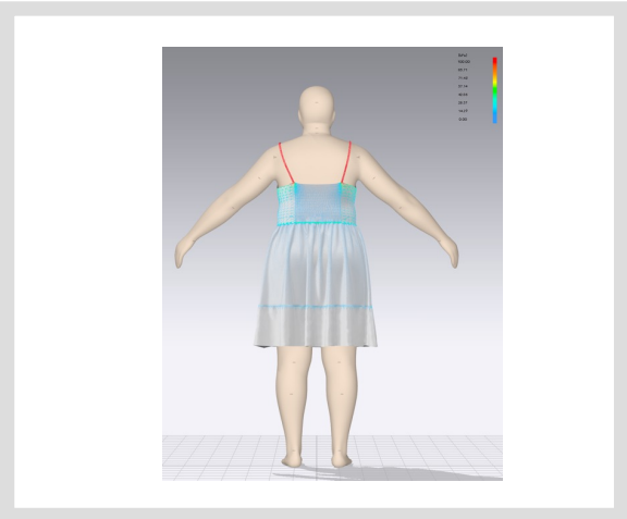
*Stress map displays the pressure of the fabric per section resulting from a tight-fitting garment
