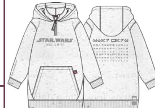
SWE23 HDFLC GRC# 106M423U094 / 106C423U094 Art Application: Embroidery, Softhand Screenprint, HD Ink, Woven Patch Fabric: Brushed Fleece - 60/40 Organic Cotton/ Recycled Poly, Flat Rib Weight: Main Body - 300GSM, 1x1 Rib - 320GSM Sizing: S-3XL
