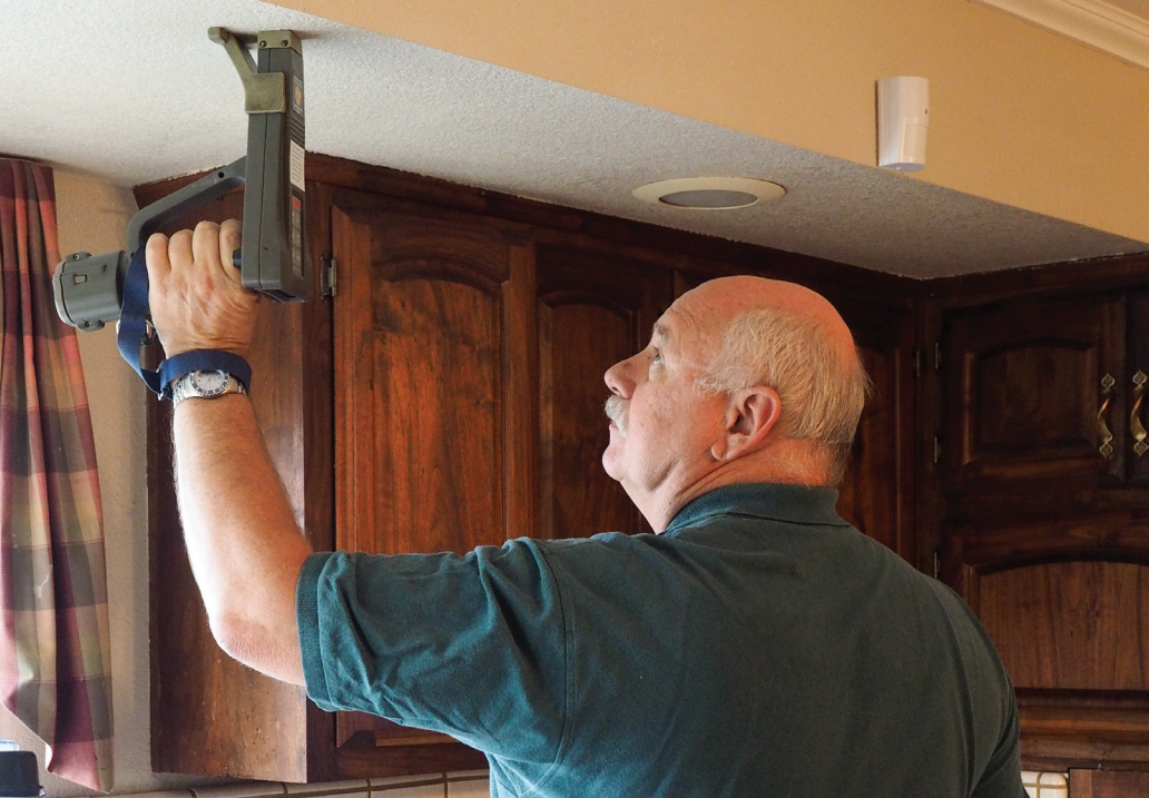
Photo by Ron Nability | Jeff Van Slooten, owner of Lead Detective Agency in Sacramento, Calif., uses an XRF analyzer to test a home for lead.
