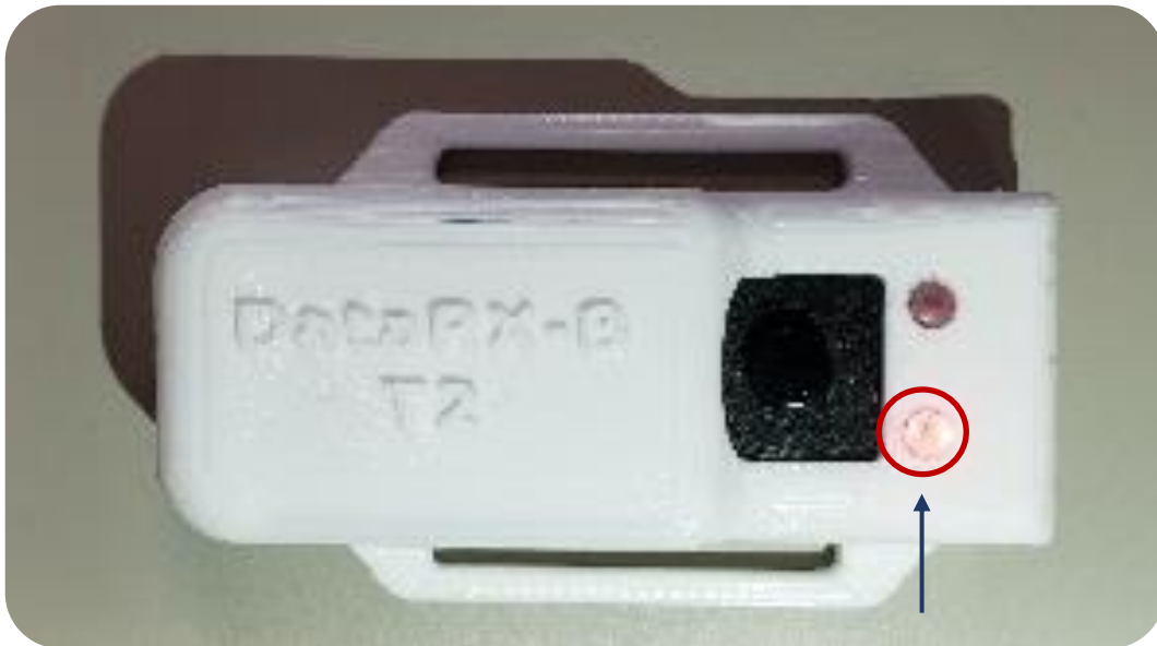
Figure 7. The Red LED blinks when the connection is not established.
