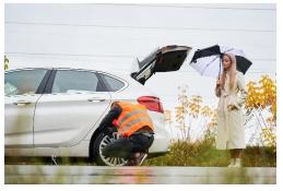
You can now remove the loosened wheel nuts and store them safely. Gripping the damaged tyre with both hands, gently pull it towards yourself until it slips off and put it to the side.
