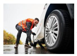
Slowly lower your vehicle to the ground and remove the jack from underneath the vehicle. Tighten the wheel nuts again using a wrench or spanner, turning clockwise as much as you can to ensure that they are as tight as possible. You can now clean up your
