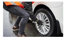
Remove the hubcap (or wheel cover) of your tyre with the flat end of the wrench. Using the wrench or spanner, you can turn the wheel nuts of the tyre anticlockwise until you loosen them up and can turn them by hand. Do not
