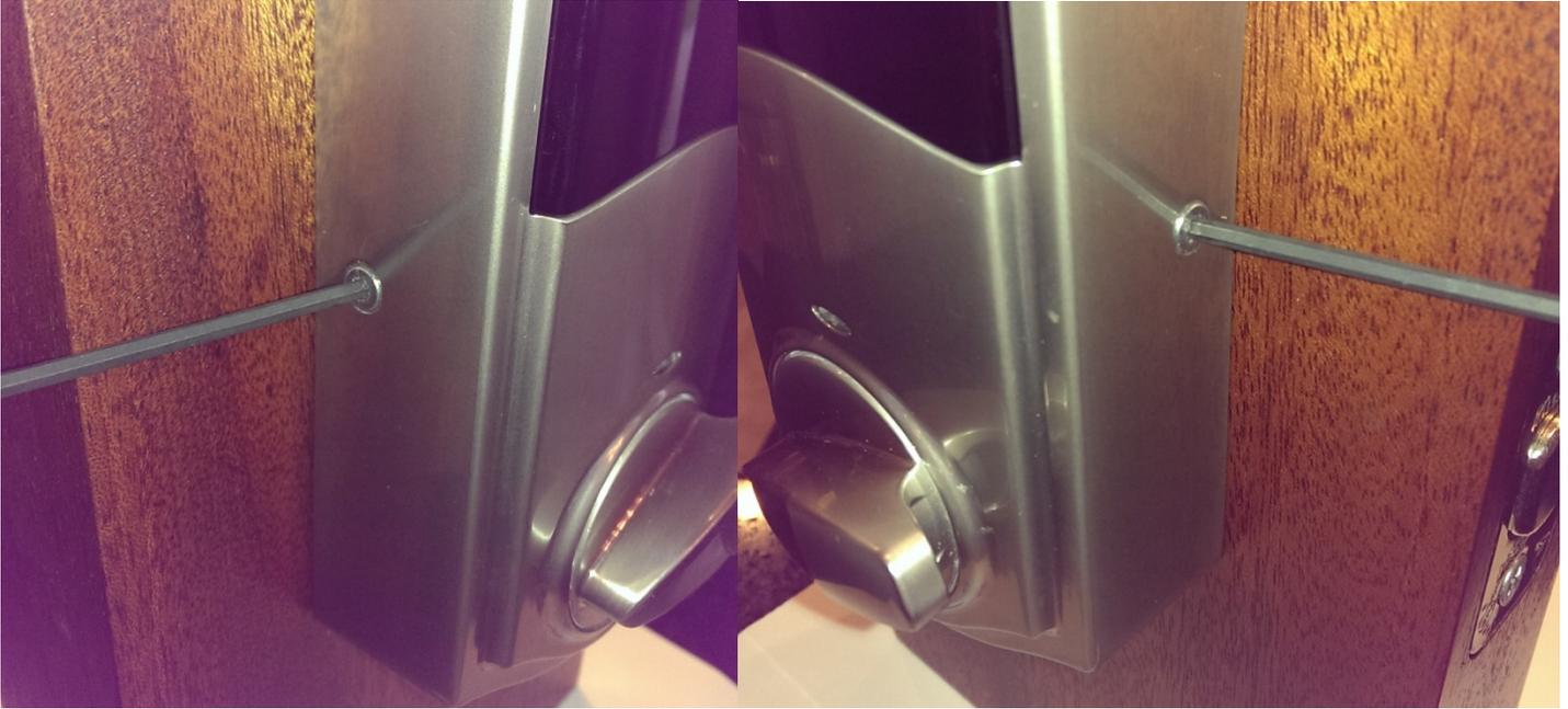
NOTE: Do not change the thumb switch position when removing the rear cover.
