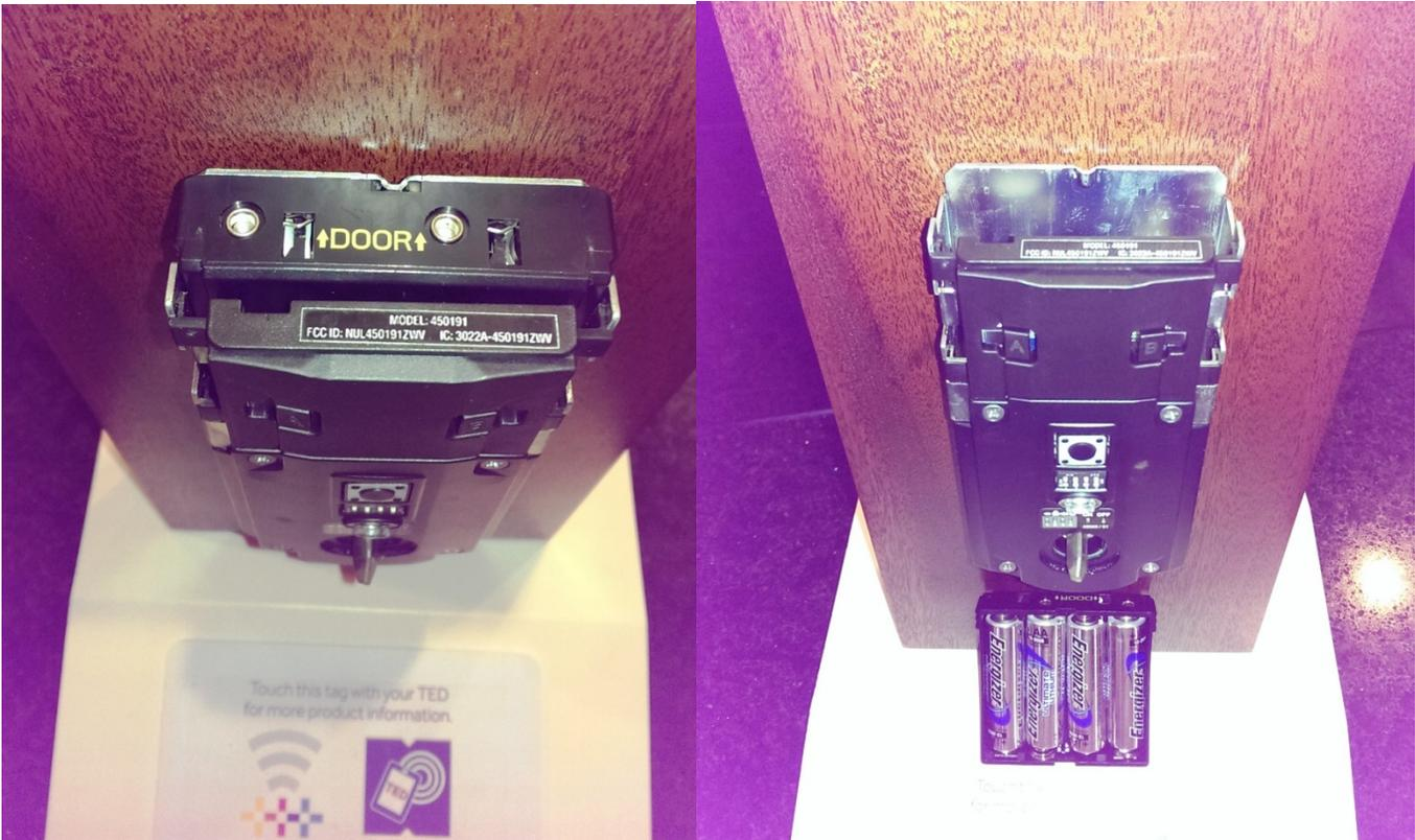
3. Remove the old batteries from the battery cartridge.
