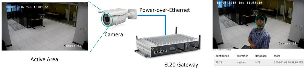
**Figure 1.** Connecting PoE camera, HPE Edgeline EL20 for face detection/recognition analytics.
