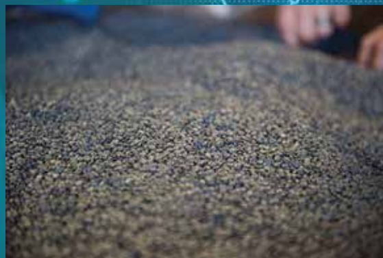
Chemical recyclers use a variety of feedstocks and methods to break plastics down to their molecular building blocks. GreenMantra uses a depolymerization process (left) to create specialty polymer additives (above) for a range of applications.
