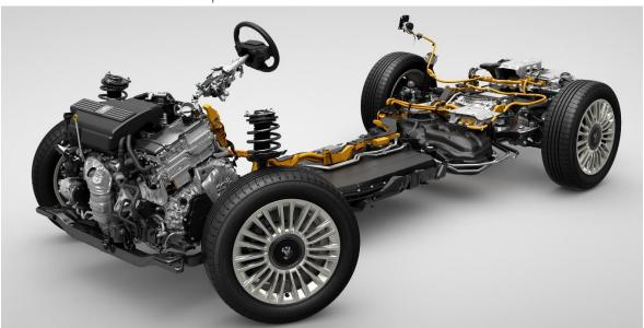
Under the hood sits a transverse-mounted 3.5-liter V6, almost half the size of the highly favored 5.0-liter V12 used in the second-generation Century. The cherry on top is that the Century SUV will be sold as a PHEV (plug-in hybrid vehicle) with an electric motor sitting on the rear axle. With an estimated weight of roughly 5,600 pounds, the electric motor sitting at the rear is an advantage.
