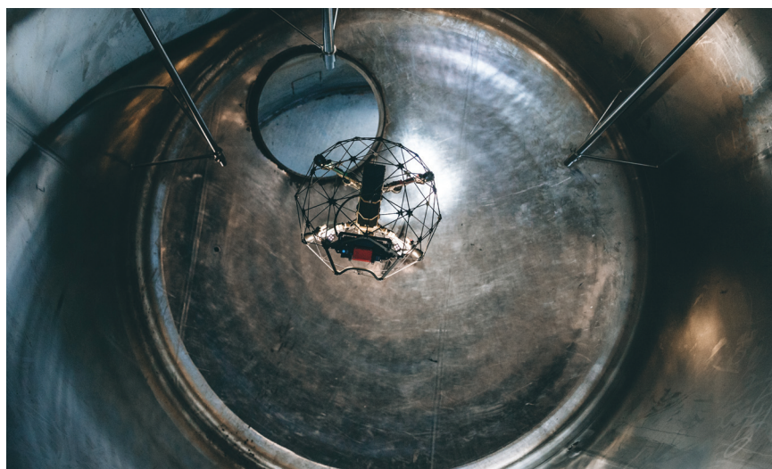
▲ ELIOS 2, a drone developed by Swiss company Flyability, is built for inspecting industrial systems. This includes oil tankers or pressure vessels. Image courtesy of Flyability.
