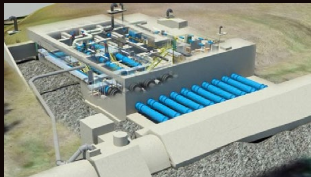
BIM data and physical scale models were used to optimise the hydraulic design of the interconnection (image courtesy of Mott Macdonald)
