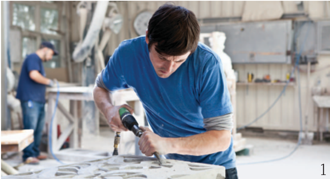
1. Hunt uses an electric chisel to carve a limestone tile. "The big difference between working with plaster and working with stone is that with stone there are no second chances," says Hunt. "With plaster, you can just add some more if you screw up." 2. A pointing machine, originally created by French sculptor Nicolas-Marie Gatteaux in the 18th century, is a measuring tool used by stone carvers to accurately reproduce sculptures from models. 3. An electron-scanning microscope helped inspire the design of these wall tiles. "It looks like a feather, but it's actually the cellular structure of a plant stem," says Hunt. 4. Master stone carver Jason Carter uses the ancient technique of pointing (covering a cast in precisely measured points) to faithfully replicate a 14th-century statue of Neptune destined for the St. Louis Museum of Art.
