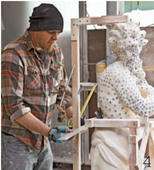
1. Hunt uses an electric chisel to carve a limestone tile. "The big difference between working with plaster and working with stone is that with stone there are no second chances," says Hunt. "With plaster, you can just add some more if you screw up." 2. A pointing machine, originally created by French sculptor Nicolas-Marie Gatteaux in the 18th century, is a measuring tool used by stone carvers to accurately reproduce sculptures from models. 3. An electron-scanning microscope helped inspire the design of these wall tiles. "It looks like a feather, but it's actually the cellular structure of a plant stem," says Hunt. 4. Master stone carver Jason Carter uses the ancient technique of pointing (covering a cast in precisely measured points) to faithfully replicate a 14th-century statue of Neptune destined for the St. Louis Museum of Art.
