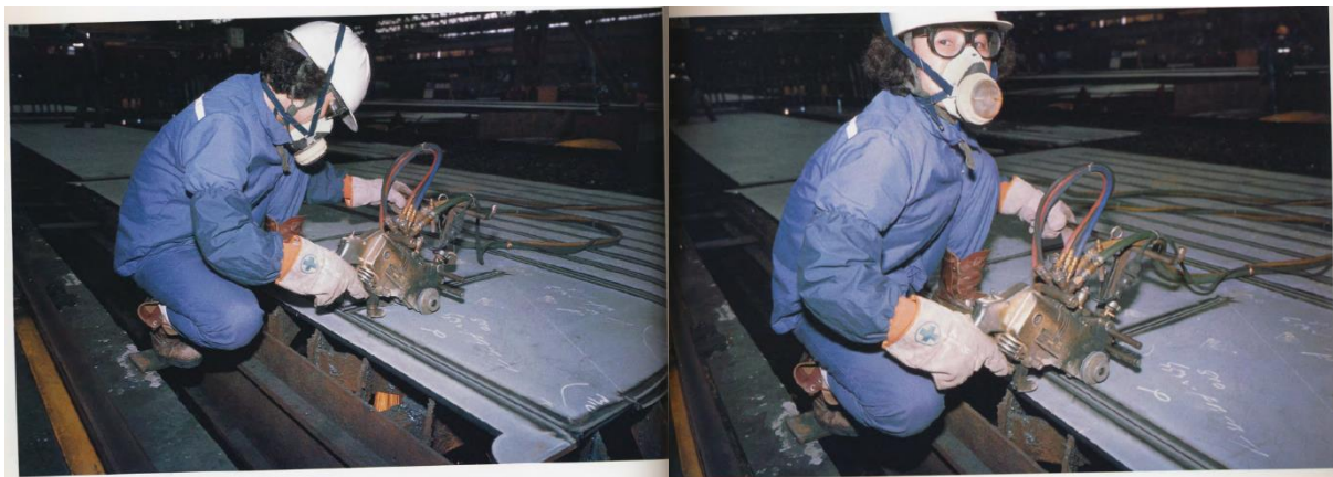
Figure 5-6: Allan Sekula, Fish Story , “Cutting steel in the plate and sub-assembly shop. Hyundai Shipyards.” South Korea. September 1993.
