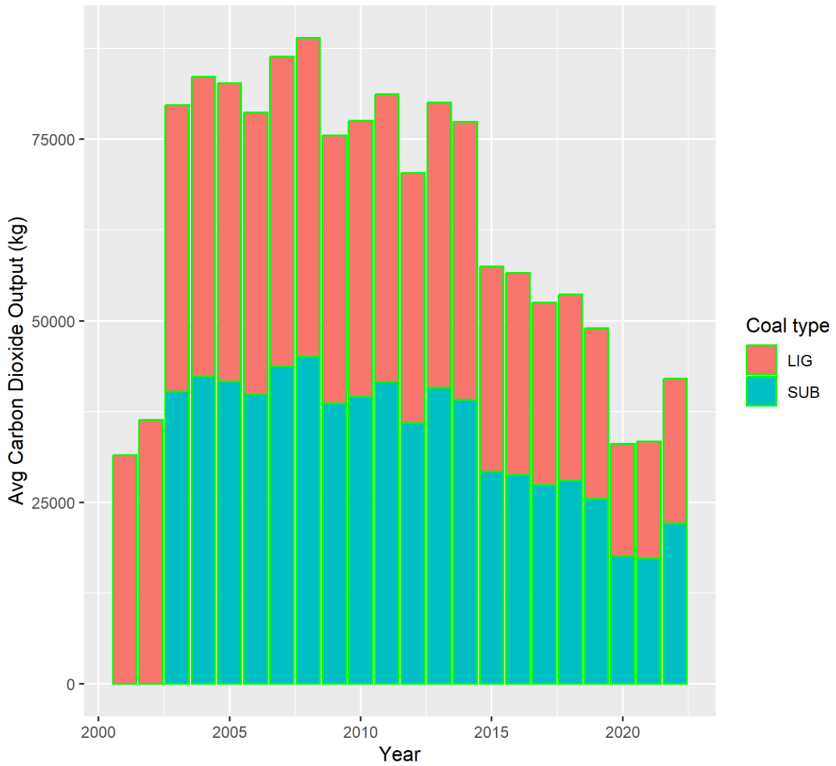
Annual Avg CO Output for Plant 298 - Limestone, Texas
