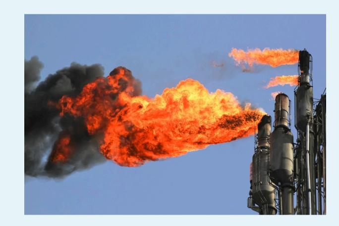
Flaring emissions during planned startups and shutdowns will typically be higher than emissions during normal operations. Flare emissions from unplanned events should not
