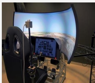
Spatial Disorientation simulator housed at NAMRU-D Spatial Disorientation lab. Specs: 130° x 60° FOV
