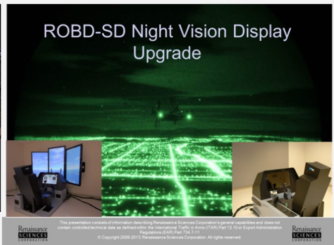
Spatial Disorientation simulator housed at NAMRU-D Spatial Disorientation lab. Specs: 130° x 60° FOV
