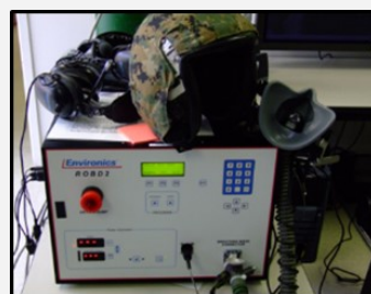
Reduced Oxygen Breathing Device (ROBD); NAMRU-D houses 6 ROBDs.
