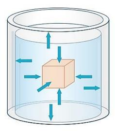
**Pressure in Liquids-** It is the thrust exerted by the liquid per unit area of an object at rest. It is a scalar quantity, with magnitude and no direction. Its dimensional formula is  $[ML^{-1}T^{-2}]$  and unit is  $N/m^2$  or Pascal (Pa).
