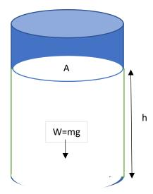
Let us consider a liquid filled till height, h in a container with surface area, A. The pressure, P exerted by the liquid on the bottom of container can be expressed as:
