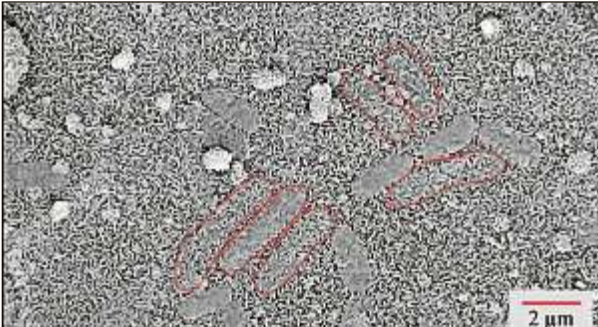
Dead and dying bacteria on an etched aluminium surface. These surfaces can be used in common areas of hospitals to prevent infections.
