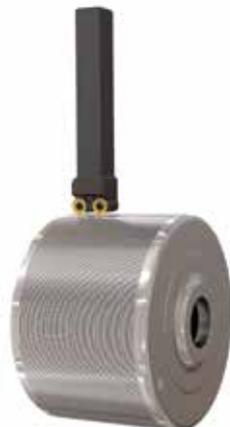
ing a combined tool with coolant holes both on top and bottom of the cutting edge to cool and blow away the chips. The two round inserts are positioned for semi finish and finishing operations, generating an excellent surface finish.
