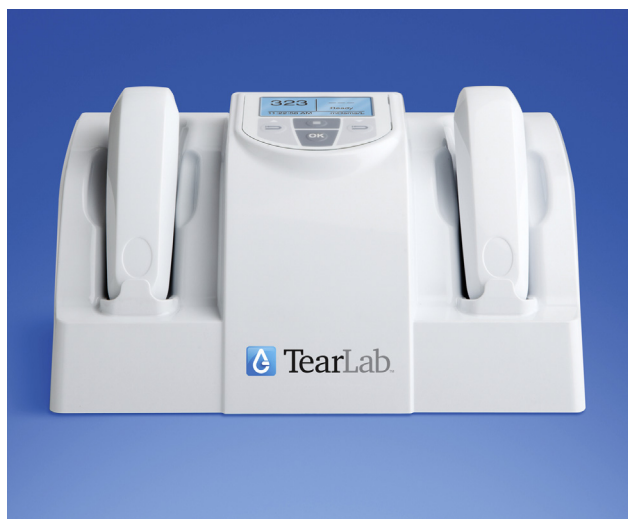
Figure IV-1. TearLab Osmometer for point of care testing. Point-of-Care testing of osmolarity provides early diagnostic and staging information. Courtesy of TearLab, Inc.
