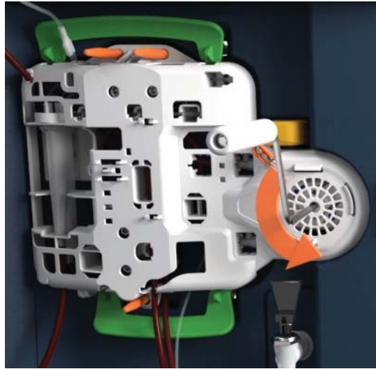
Figure 57. Place Hand-Crank in Far Right Hole of Cartridge
