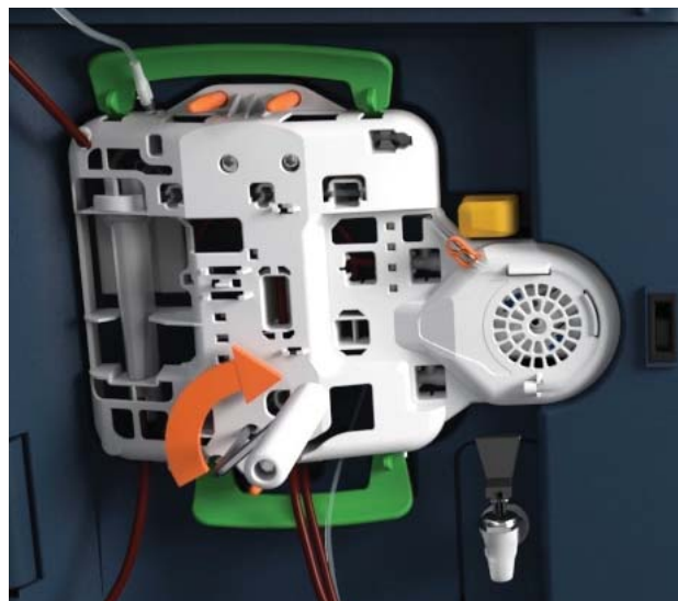
Figure 51. Place Hand-Crank in Bottom Hole of Cartridge
