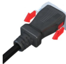
Figure 12. Detaching Power Cord from System
