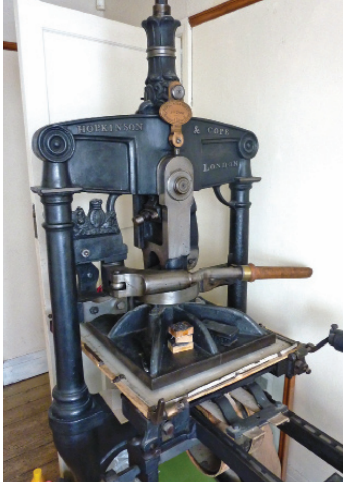
The Albion platen press, manufactured in the 19th century by Hopkinson and Cope of Finsbury, London
