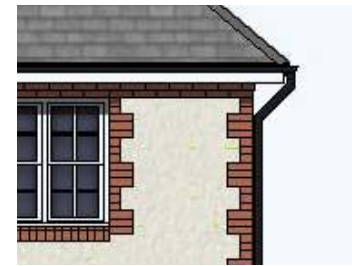
> Contrasting brick quoins
