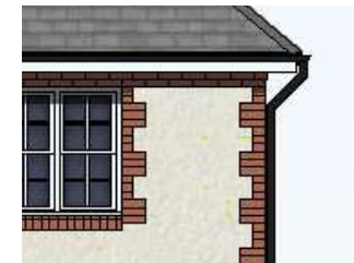
> Contrasting brick quoins
