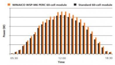
Differences in energy output across a whole day between WINAICO's PERC module and a standard solar module.
