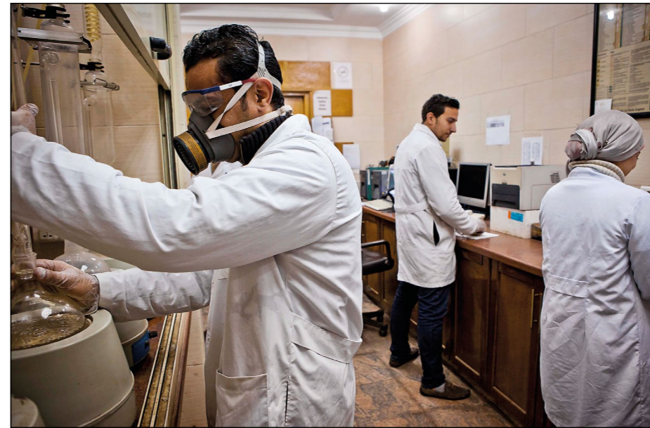
..... Careful preparation of samples, including extraction of unwanted organic matter, mud additives or well-site contaminants, is often necessary to achieve the most accurate possible geochemical analyses.
