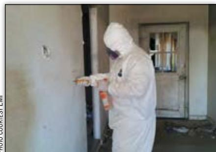
Outfitted in protective clothing, a technician prepares to take a sample to test for asbestos contamination. Asbestos was used in textured paint and patching compounds on walls and ceiling joints in structures built before 1980. Its use was highly regulated in 1977.
