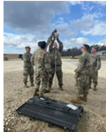
Soldiers from the 578th FES practice using the dynamic cone penetrometer
