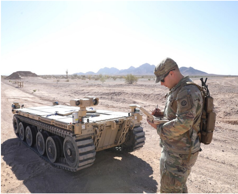
Army Pfc. Daniel Candales uses a tactical robotic controller to control an expeditionary modular autonomous vehicle as a practice exercise in preparation for Project Convergence at Yuma Proving Ground, Ariz., Oct. 19, 2021. Project Convergence is the Army's contribution to the military-wide Joint All Domain Command and Control concept, where data will link together land, air, sea, cyber and space capabilities.
