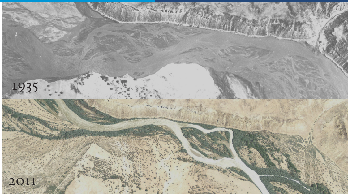
Aerial photos from 1935 (top) and 2011 (bottom) show how the side channels of the San Juan River dried up over time because of limited runoff from the Navajo Dam and invasive tree growth. © Soil Conservation Service/USDA
