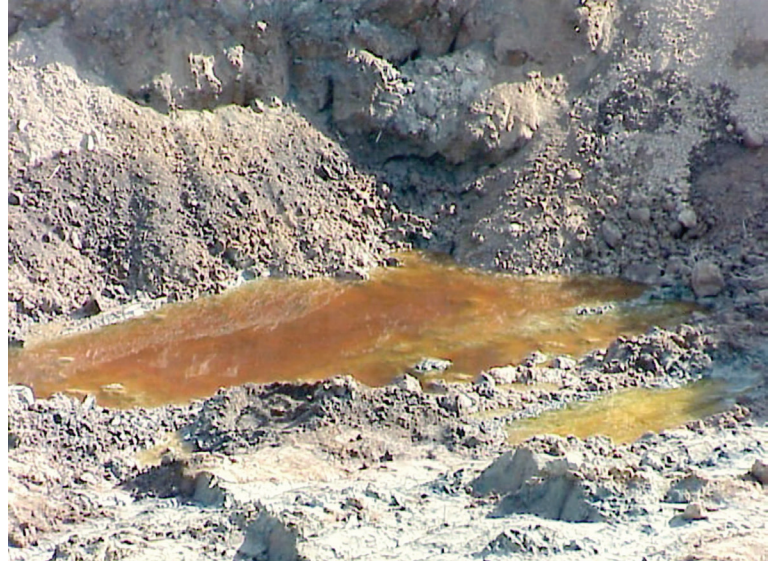
LEFT: Flooding and poor drainage plagued K2, including the area around the mess station. Sandbags were filled with contaminated dirt. RIGHT: An Army environmental survey team found a pool of jet fuel 8 feet below the surface, the result of fuel tanks at the former Soviet base that had leaked for 30 years. Photos courtesy Mike Lechlitner
