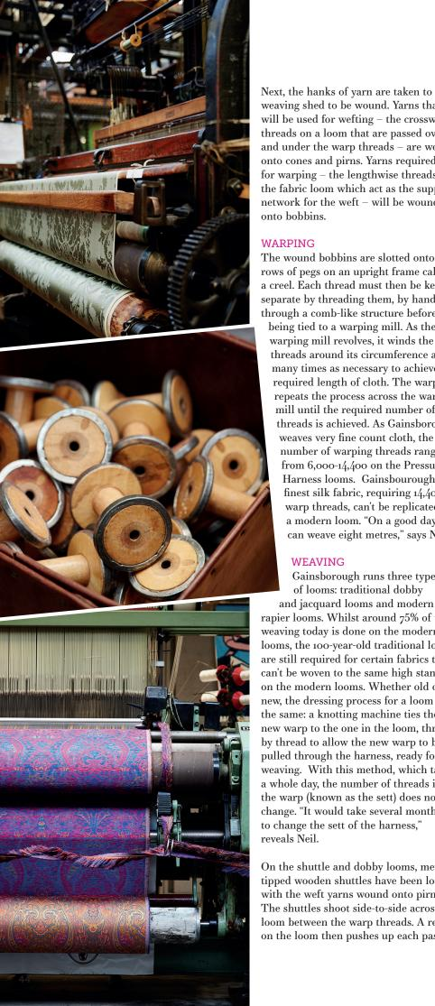
Next, the hanks of yarn are taken to the weaving shed to be wound. Yarns that will be used for wefting - the crosswise threads on a loom that are passed over and under the warp threads - are wound onto cones and pirns. Yarns required for warping - the lengthwise threads on the fabric loom which act as the support network for the weft - will be wound onto bobbins.
