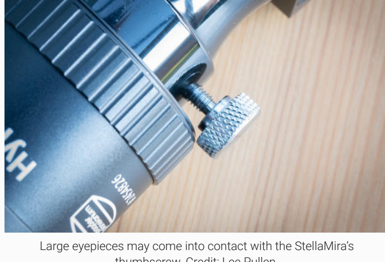
Large eyepieces may come into contact with the StellaMira's thumbscrew. Credit: Lee Pullen.
