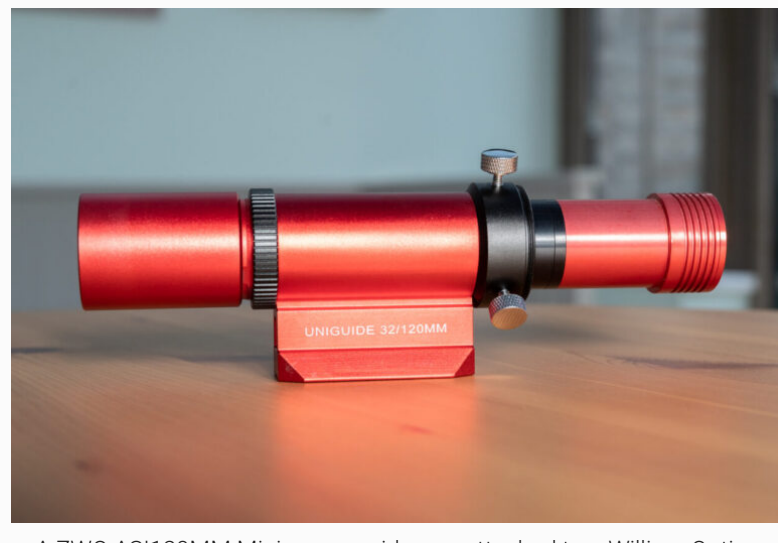
A ZWO ASI120MM Mini mono guidecam attached to a William Optics 32mm Slide-base Uniguide Scope. Credit: Lee Pullen.
