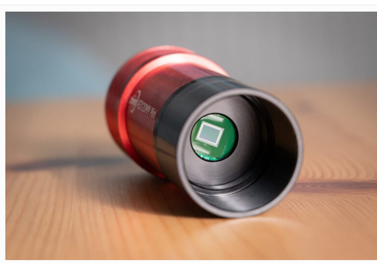
The ZWO ASI120MM Mini mono sensor size is small, but perfectly adequate for guiding. Credit: Lee Pullen.
