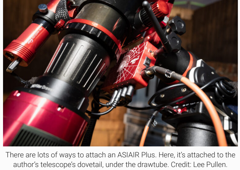
There are lots of ways to attach an ASI AIR Plus. Here, it's attached to the author's telescope's dovetail, under the drawtube. Credit: Lee Pullen.
