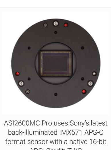
ASI2600MC Pro uses Sony's latest back-illuminated IMX571 APS-C format sensor with a native 16-bit ADC. Credit: ZWO
