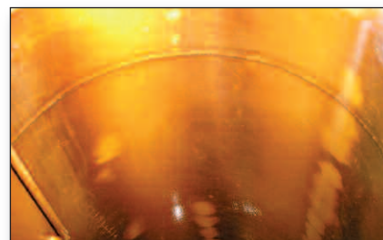
Filter housing internals coated with varnish
