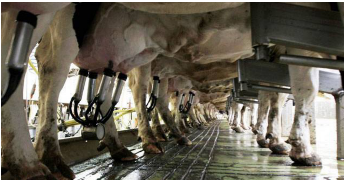
The automatic milking parlor at Al Rawabi. The machine consists of four teat cups, a long tube and a pulsator.
