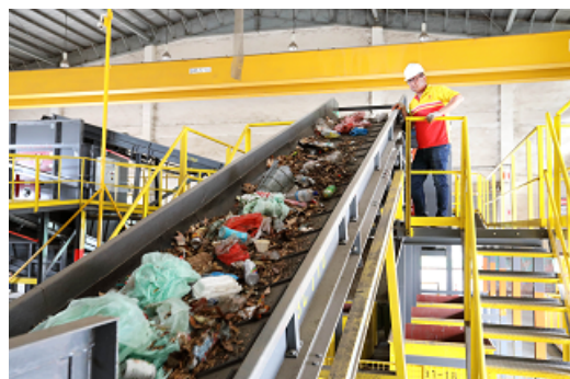
CTM's semi-automatic sorting system separates paper, leaves, plastics, glass bottles and nonferrous metals that are recovered for further use.
